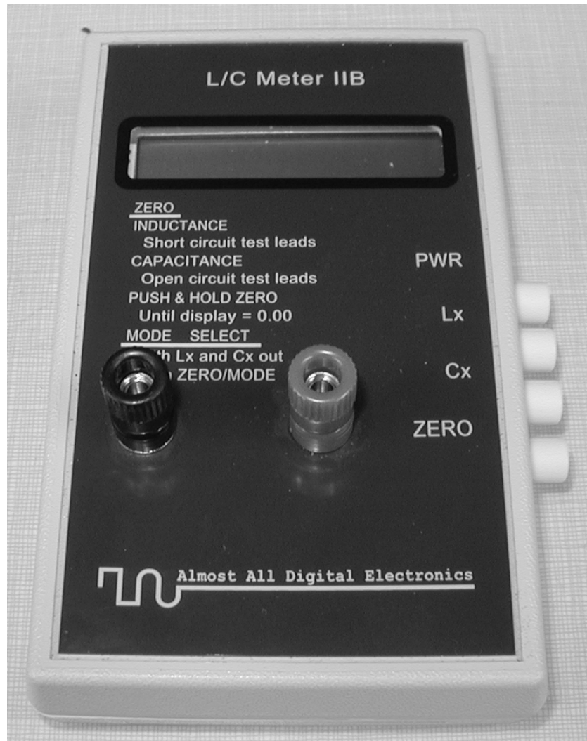
Figure A1, L/C meter
