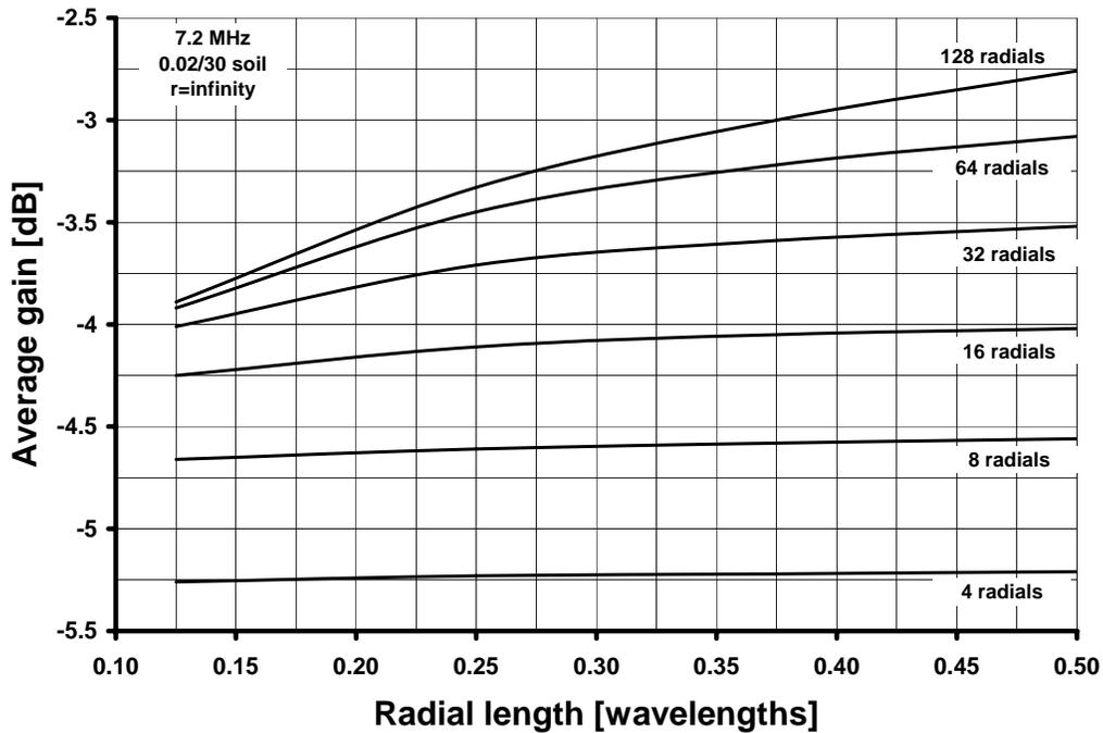
Figure 4, Efficiency in terms of **Ga** for very good soil.
