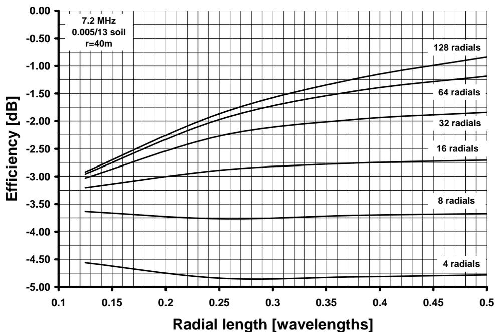
Figure 1, efficiency in dB as a function of radial number and length in average soil. **r**=40 m.
