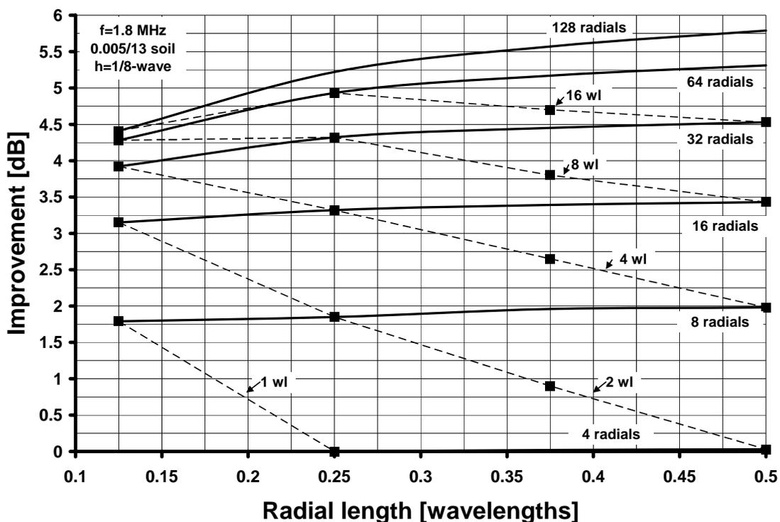
Figure 5, improvement in dB for various radial combinations for a 1/8-wave vertical.
