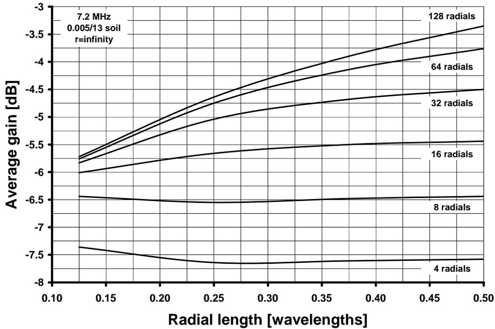
Figure 3, Efficiency in terms of **Ga** for average soil.
