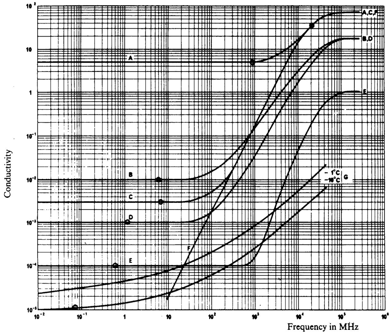
Fig. 3.1 Permittivity  $\epsilon$  and conductivity  $\sigma$  of the Earth's surface: A: sea water (mean salinity), 20°C; B: humid soil; C: fresh water, 20°C; D: moderately dry soil; E: very dry soil; F: pure water, 20°C; G: ice (fresh water); ring: transition frequency.
