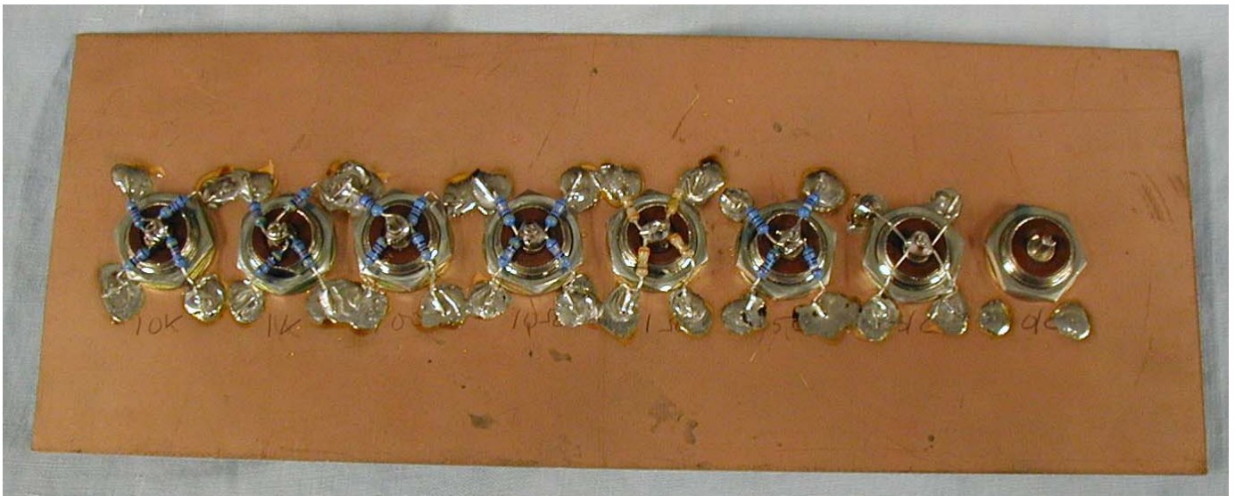
Figure 1B, VNA calibration board rear view
