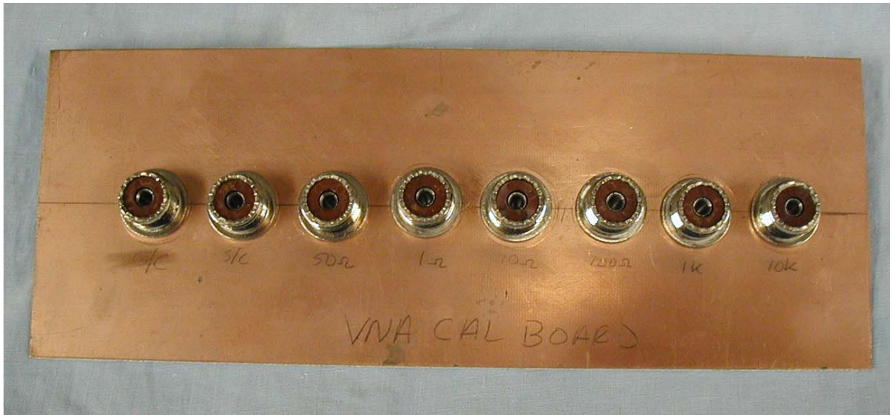
Figure 1A, VNA calibration board front view
